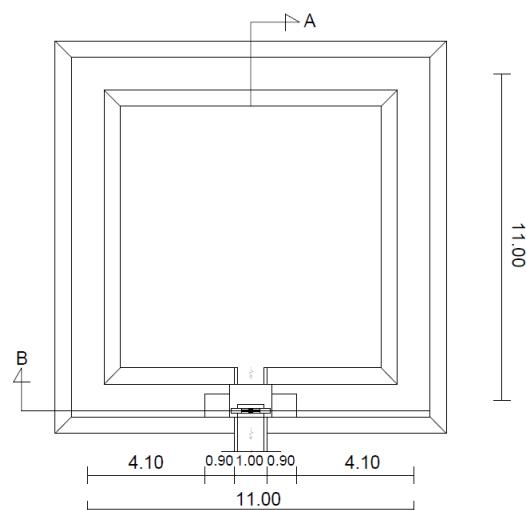
**Gambar 4.** Denah Embung Serbaguna.
