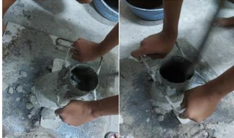
**Gambar 6** Uji Slump
