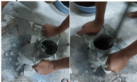
**Gambar 6** Uji Slump
