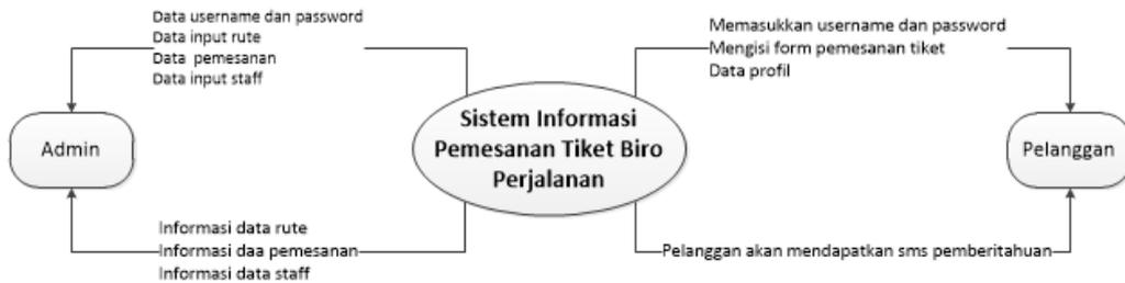
Gambar 3. *Data Flow Diagram Level 0* (Konteks Diagram)
