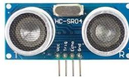
Gambar 3. Sensor Ultrasonic HC SR04
