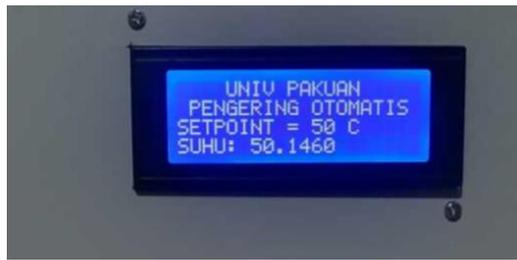
Gambar 17. Sensor Suhu Mendeteksi Temperature Heater
