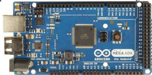
Gambar 1. Arduino Mega
