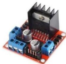
Gambar 5. Modul Driver Stepper Motor *L298N*
