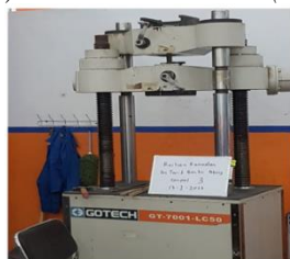
Gambar 7 Universal Testing Machine/UTM Sumber: Dokumentasi , (2023)
