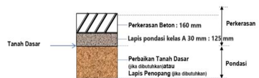
Gambar 4. Rencana Lapis Perkerasan Kaku (Rigid Pavement)
