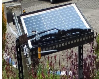
Gambar 4. Panel surya kondisi tanpa debu
