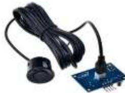
Gambar 4. Sensor jarak JSN-SRT04
